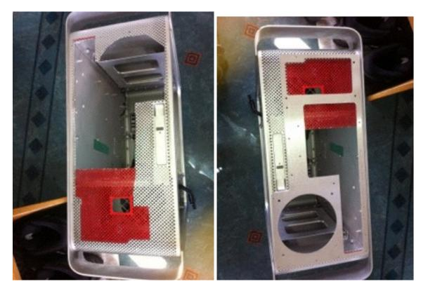
Start by masking the area where you will be cutting and using a rotary tool (e.g. Dremel) cut out the original IO section.
