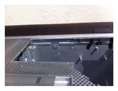
Carefully check around where the PCI slots were and remove any traces of them - remaining parts where the slots were welded in place can be removed using a small screw driver from inside the case.
