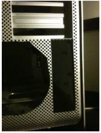
You need to remove the PCI slots and this is probably one of the hardest parts - start by cutting around the slots like this you MUST keep one row of holes as marked by the green box:
