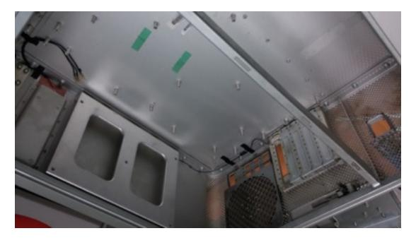
If your Mac Pro has an internally fastened lower shelf as shown in the photo above (i.e. a shelf at the bottom of the case with a support as shown) then this lower shelf support must be removed.
