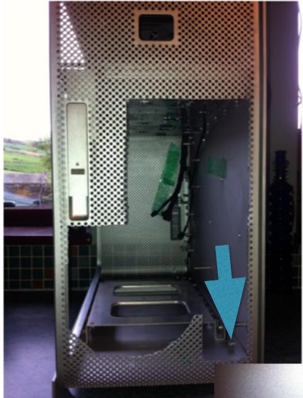
The four rear most of the lower case screws mounting pointsi.e. referring to the photo to the right, the blue arrow indicates one of the case screw mounts.
