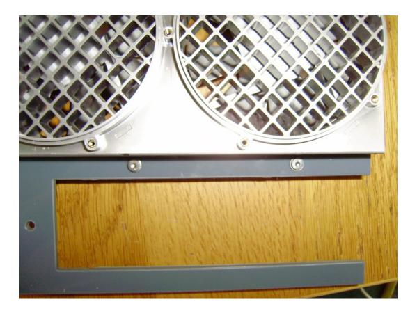
10. You have now finished all the adaptations to the back of the G5 and can fix the main backplate into position tightly with the countersunk screws and nyloc nuts provided. If however you are going to now fit the motherboard tray do not put the fan assembly into position yet.
