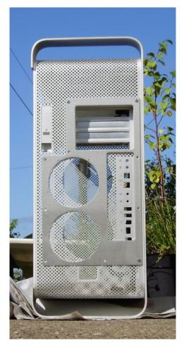
4. The Picture below shows an example of the material to be cut away. Note that the mesh needs to be cut right up to the wall of the PCI compartment, one full column of holes needs to be left on the right hand side and five colums of holes on the left hand side.
