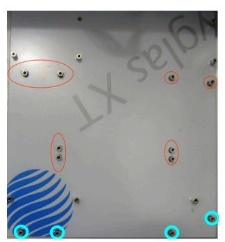
3. For a few G5s, you may find you need to attach the motherboard tray to standoffs that are inside the footprint of the ATX motherboard. For instance, in the motherboard tray shown below, the tray had to be attached at the points arrowed. For these two mount points the standoffs had to be reduced in size by the use of a dremel tool or hacksaw so that when the motherboard was mounted to the tray there was no chance of them interfering with it.
