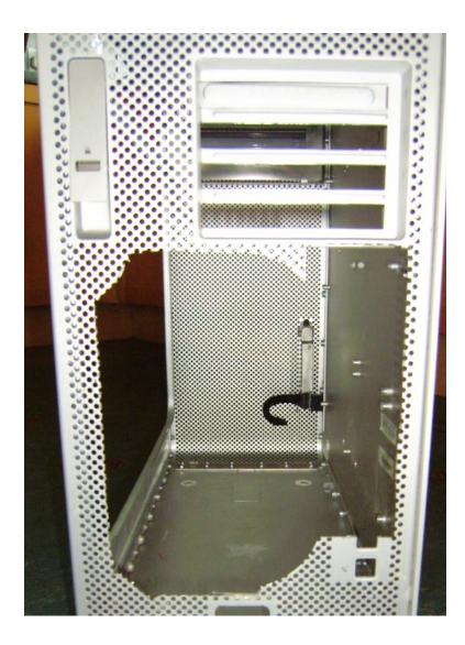
6. Once you have made the cuts test fit the new back. This time, once you have loosely fastened the new back plate into place offer up the G5 fan plate (with the tongue facing inwardly - i.e. the opposite way to the original G5 fitment) to the rear of it and see if all fits well. If there is too much of the original back to allow the fan assembly to fit, then make a note of where the problem is, take the backplate off and do any needed extra cutting.
