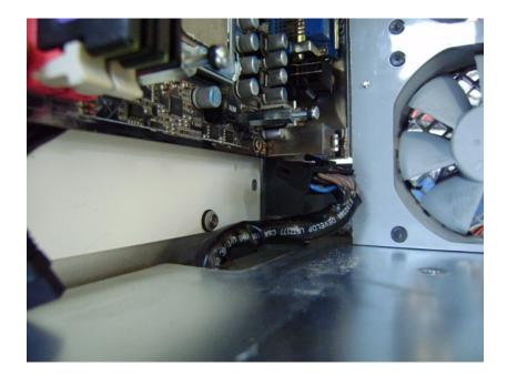
Loosely associate the metal I/O shield with the rear ports of the mobo and feed the mobo into position on the tray.
